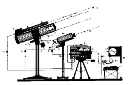
AC-rendition (for AC recording) of the data envelope modulated by a DC amplifier, and final recording of data by a field recorder. A processing amplifier and meter provide primary, unmodulated monitoring of the incoming signals.
